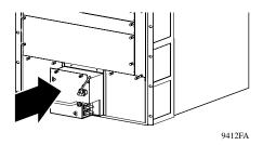
3. Push the power supply partway into the bay. Leave the terminal block at the side of the power supply exposed.
